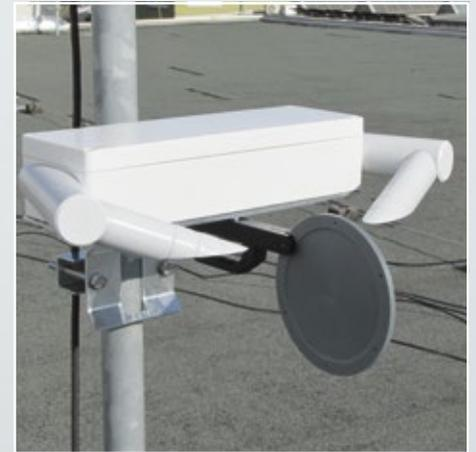
Verification in the field is carried out using a calibration disc. As a further control point, the zero point is checked ("in the dark").
