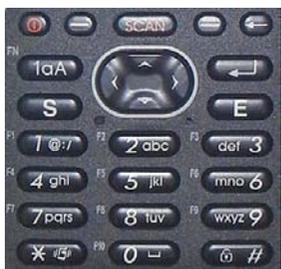
physical keypad, and it can be used for entering text as well. It's an expanded cellphone layout with some additional keys. The numeric keys that also access numbers, letters and symbols can also be used as function keys, all the way from F1 to F10. No consumer phone can do that.
