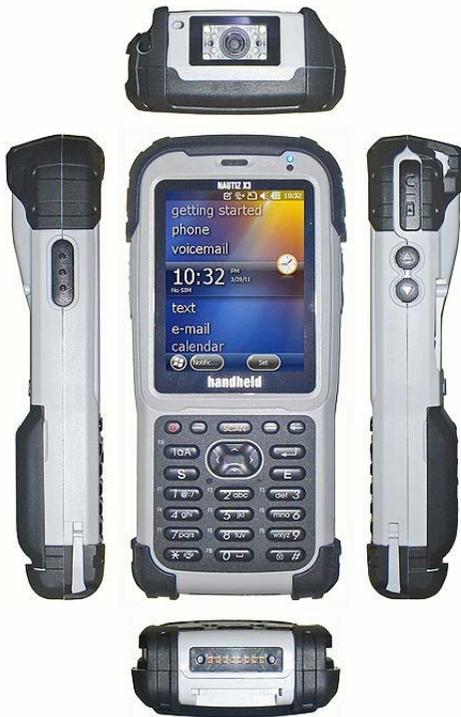
The design of the housing is elegant, clean and functional. There are hardly any visible screws and no small parts or details that look like they could break off. The entire device feels solid and capable of standing up to hard use. Note that the black bumpers serve as design elements as well as for protection. They seem glued on and it's not clear if they are meant to be replaceable should they get damaged.
