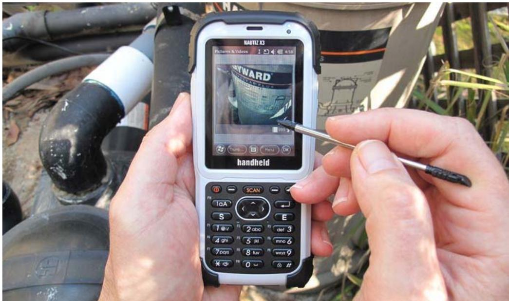
The sunlight-readable display measures 2.8 inches diagonally—a bit small perhaps considering that even tiny cameras now have 3-inch displays and larger and the trend in smartphones has been 3.5-inch and larger. It's a conventional resistive touchscreen that can be operated with a finger or the supplied stylus. The backlit 22-key phone-style keypad with smaller alphanumeric lettering includes a navigation diamond as well as ten(!) function keys and a dedicated scan key.
