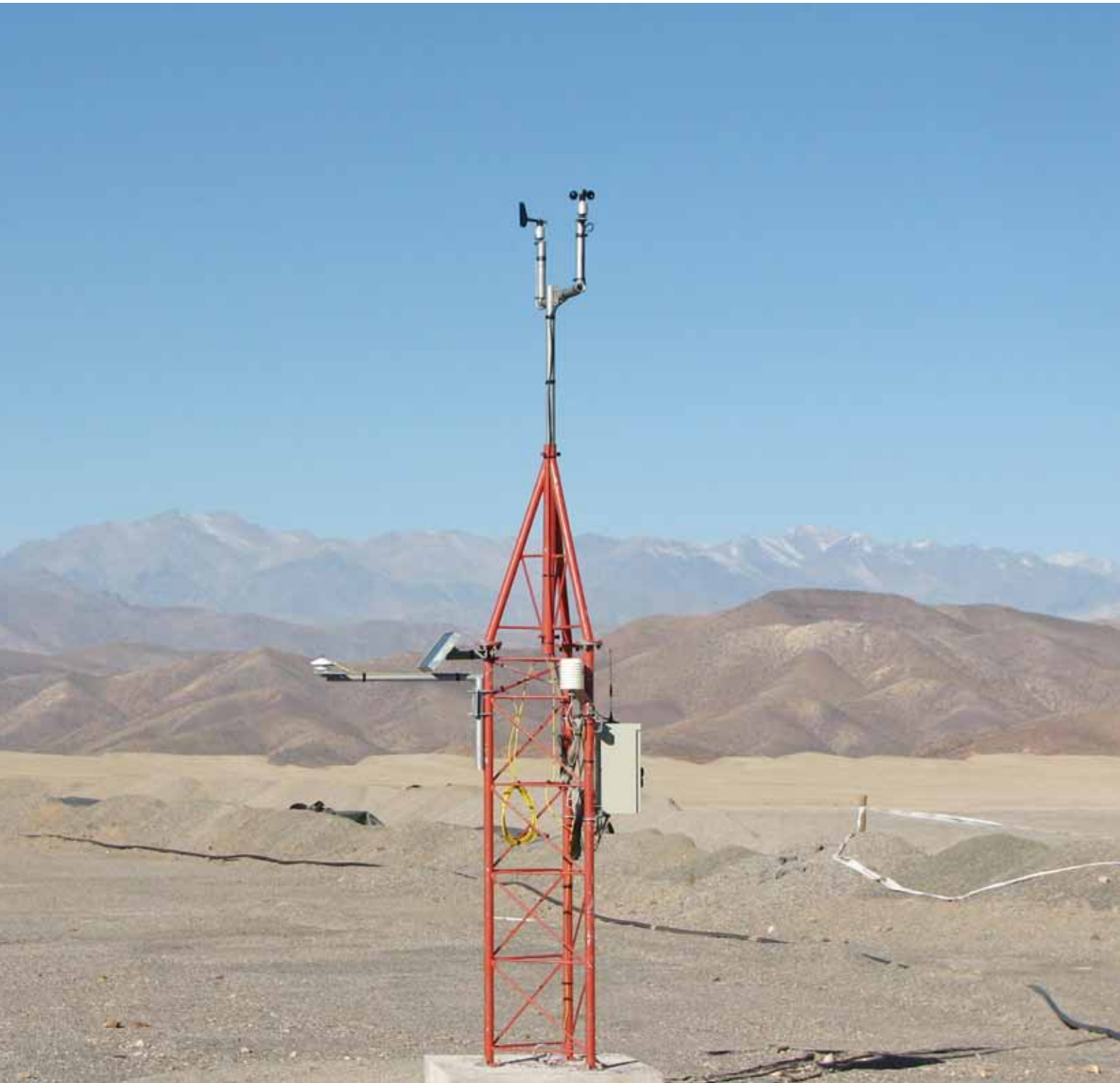
© Ammonit / DesamD (Ammonit partner Chile): typical solar measurement system in Northern Chile
